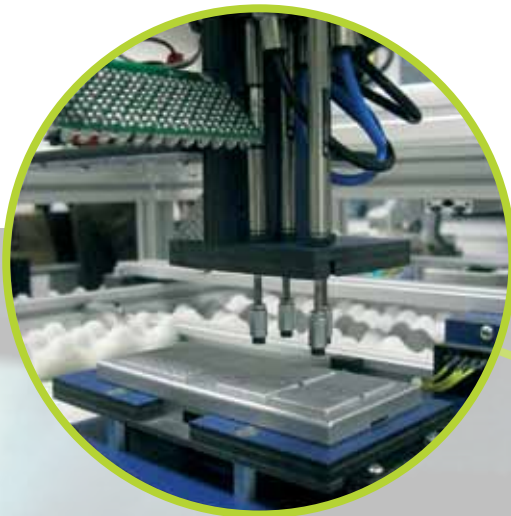
Pneumatic push fingers operate the keys of the specimen during the test.
