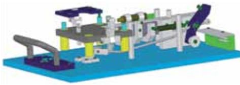
Adaptation as exchange unit with lever mechanics
