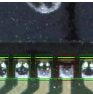
QFN with soldering defect
